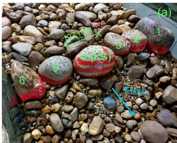
Figure 2: Flume experiment settings in Zhang et al., (2020): (a) the artificially built-up step-pool model using natural stones, with stone number labelled; (b) the unsteady hydrograph of the run ofused in this study . KS in (a) is short for keystone and DCI in (b) is discharge change interval. The run index in (b) is CIFR (continually-increasing-flow-rate) T2-used-in-this-study.
