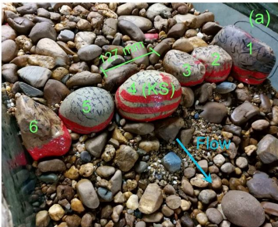
125 Figure 2: Flume experiment settings in Zhang et al., (2020): (a) the artificially built-up step-pool model using natural stones, with stone number labelled; (b) the unsteady hydrograph of the run used in this study. KS in (a) is short for keystone and DCI in (b) is discharge change interval. The run index in (b) is CIFR (continually-increasing-flow-rate) T2.
