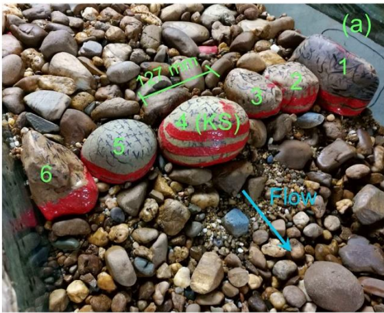
Figure 2: Flume experiment settings in Zhang et al., (2020): (a) the artificially built-up step-pool model using natural stones, with stone number labelled; (b) the unsteady hydrograph of the run used in this study. KS in (a) is short for keystone and DCI in (b) is discharge change interval. The run index in (b) is CIFR (continually-increasing-flow-rate) T2.
