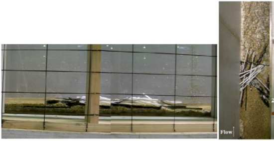
Figure 4: Log jam formation in run 15; the Itoh et al. (2010) experiment
