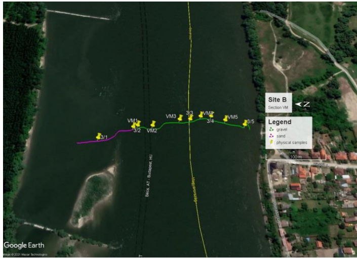
517 518 Figure 1016: The path of the vessel and camera in Section VM, Site B. The polyline is coloured based on the sediment 519 seen during visual evaluation of the video. Yellow markers are the locations of physical bed material samplings. (Map 520 created with Google Earth Pro)
