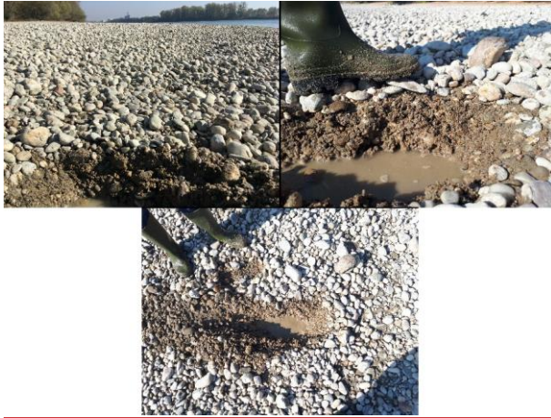
493 Figure 12: Images of bed armoring, taken during our surveys in the Upper section of the Hungarian Danube.
