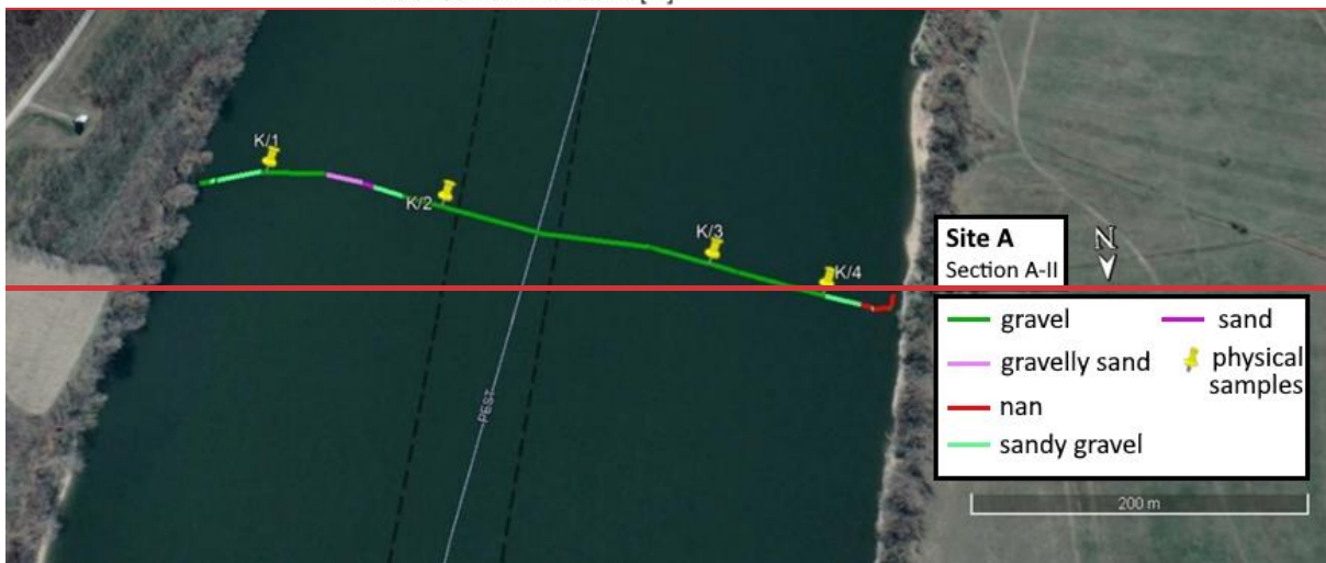
Figure 77: a) The path of the vessel and camera in Section A – II, Site A. The polyline is coloured based on the sediment features seen during visual evaluation of the video. Yellow markers are the locations of physical bed material samplings. (Map created with Google Earth Pro). b) The visual evaluation of the dominant sediment features in the video (top) compared to sediment fraction percentage, recognised by the DL algorithm (bottom). DL result after applying moving-averaging. The visual evaluation included four classes: gravel – G, sandy gravel – sG, gravelly sand – gS, sand – S.). The fractions of the physical samples are shown as verticals.
