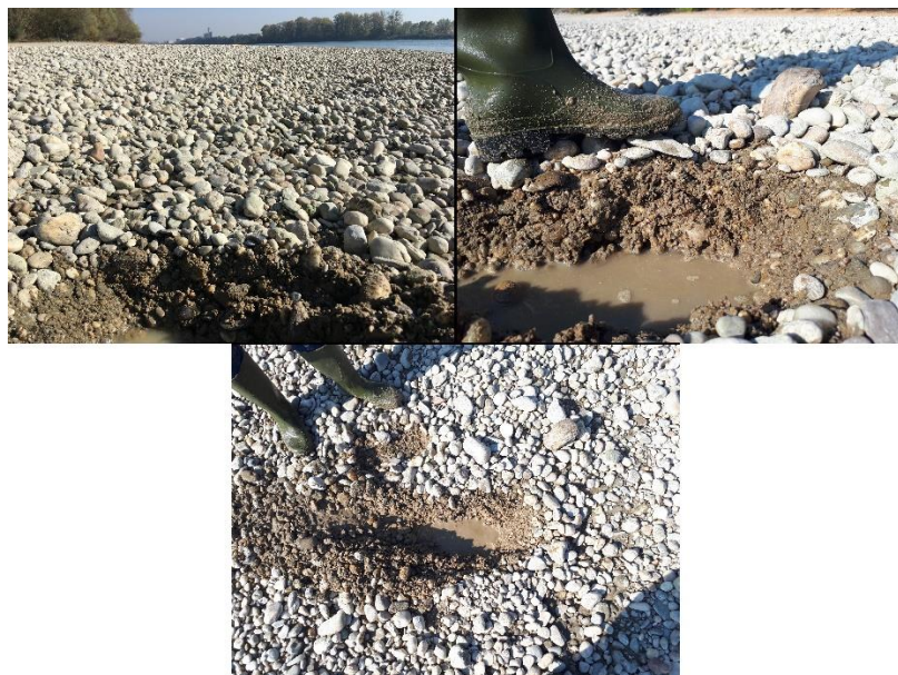
Figure 11: Images of bed armouring, taken during our surveys in the Upper section of the Hungarian Danube.
