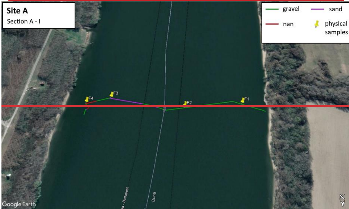
Figure C1A1: The path of the vessel and camera in Section A - I, Site A. The polyline is coloured based on the sediment seen during visual evaluation of the video. Yellow markers are the locations of physical bed material samplings. (Map created with Google Earth Pro)
