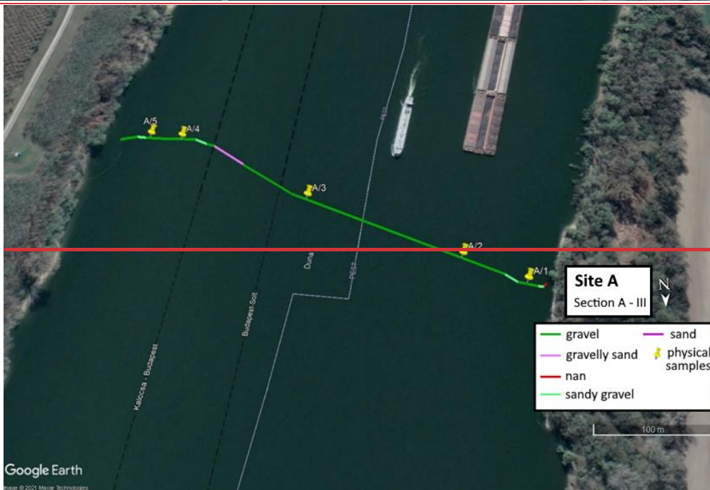
Figure DB1: The path of the vessel and camera in Section A - III, Site A. The polyline is coloured based on the sediment seen during visual evaluation of the video. Yellow markers are the locations of physical bed material samplings. (Map created with Google Earth Pro)
