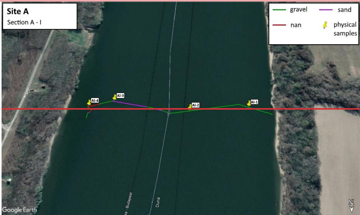
Figure C1: The path of the vessel and camera in Section A - I, Site A. The polyline is coloured based on the sediment seen during visual evaluation of the video. Yellow markers are the locations of physical bed material samplings. (Map created with Google Earth Pro)
