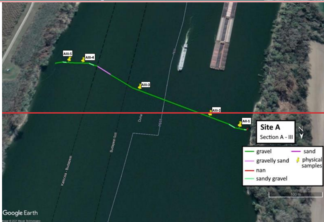
Figure D1: The path of the vessel and camera in Section A - III, Site A. The polyline is coloured based on the sediment seen during visual evaluation of the video. Yellow markers are the locations of physical bed material samplings. (Map created with Google Earth Pro)
