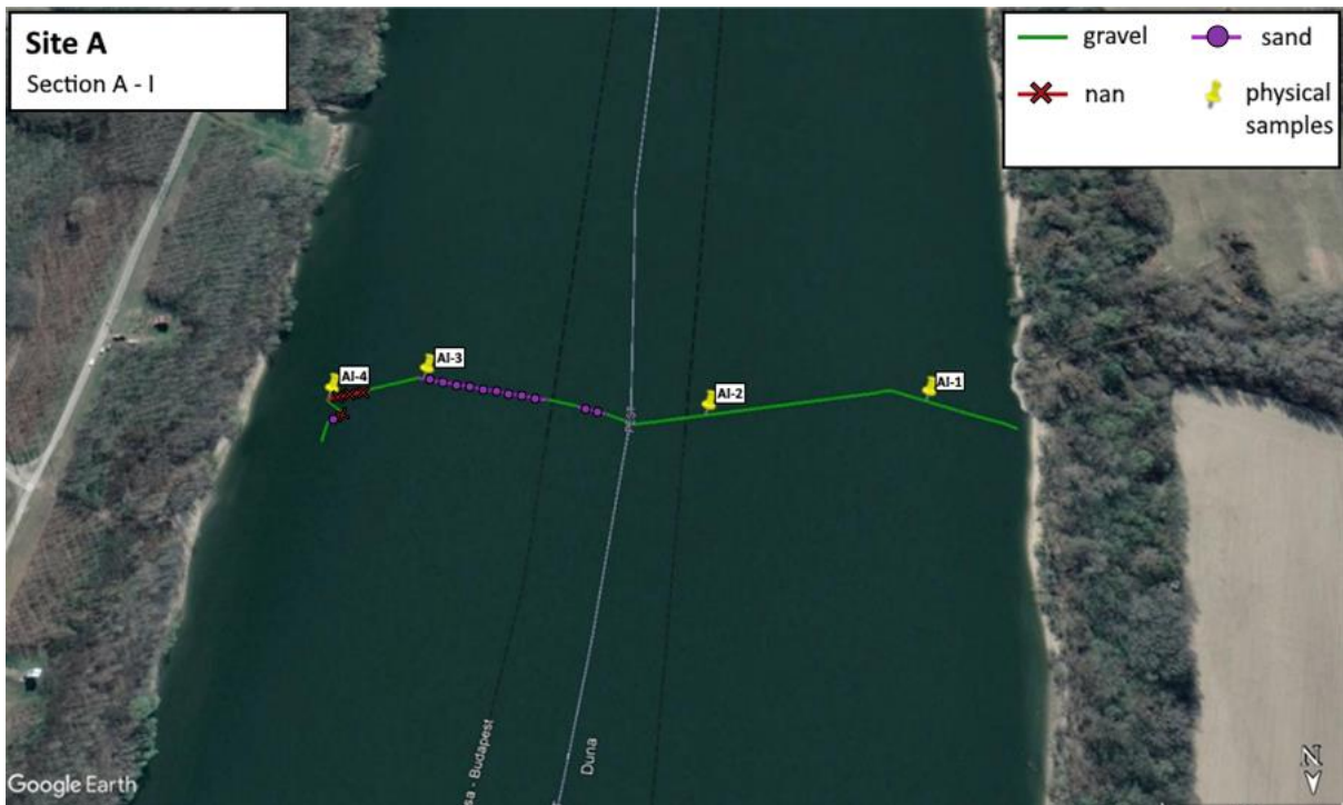
1196 Figure C1: The path of the vessel and camera in Section A - I, Site A. The polyline is coloured based on the sediment 1197 seen during visual evaluation of the video. Yellow markers are the locations of physical bed material samplings. (Map 1198 created with Google Earth Pro) 1199
