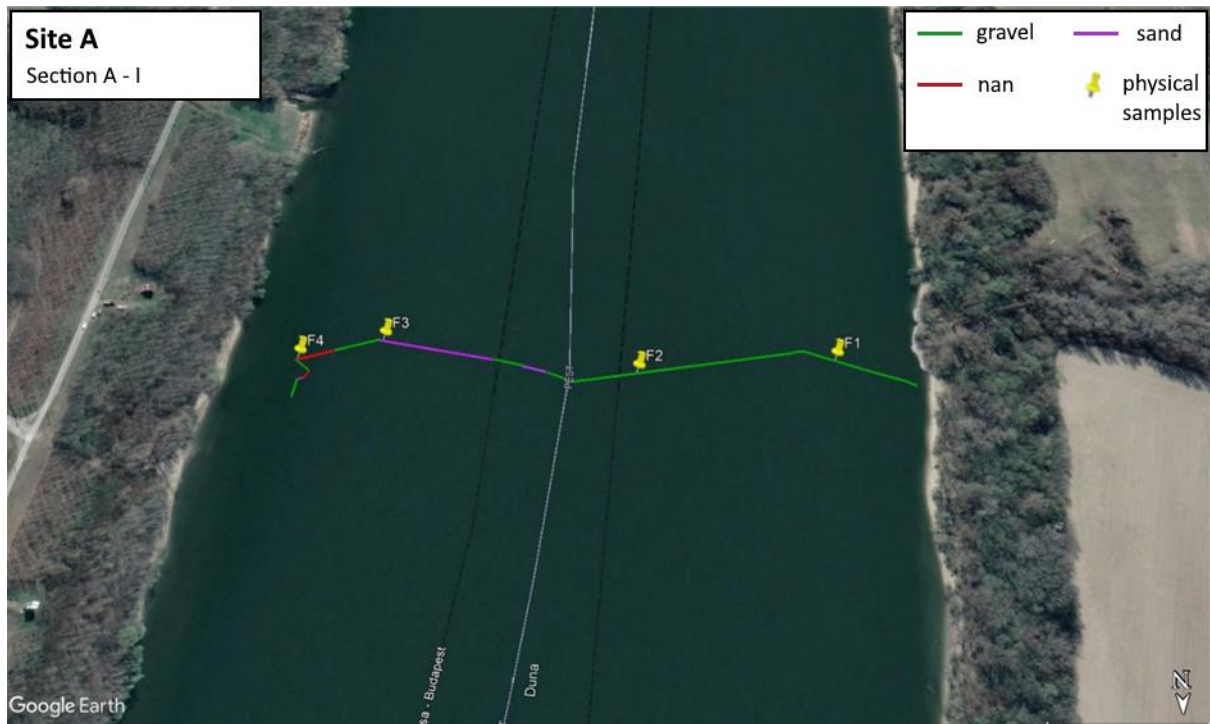
1063 Figure A1: The path of the vessel and camera in Section A - I, Site A. The polyline is coloured based on the sediment 1064 seen during visual evaluation of the video. Yellow markers are the locations of physical bed material samplings. (Map 1065 created with Google Earth Pro) 1066
