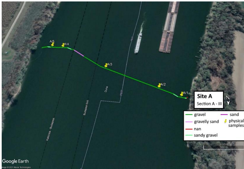
1082 1083 Figure B1: The path of the vessel and camera in Section A - III, Site A. The polyline is coloured based on the sediment 1084 seen during visual evaluation of the video. Yellow markers are the locations of physical bed material samplings. (Map 1085 created with Google Earth Pro)
