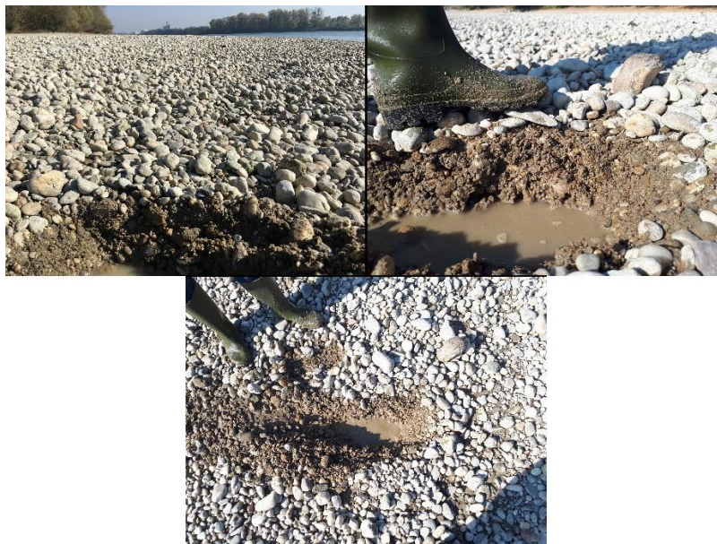
Figure A2: Images of bed armouring, taken during our surveys in the Upper section of the Hungarian Danube. We broke the surface armour to showcase the presence of the underlying finer fractions.
