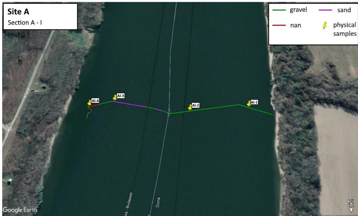
1095 Figure C1: The path of the vessel and camera in Section A - I, Site A. The polyline is coloured based on the sediment 1096 seen during visual evaluation of the video. Yellow markers are the locations of physical bed material samplings. (Map 1097 created with Google Earth Pro) 1098
