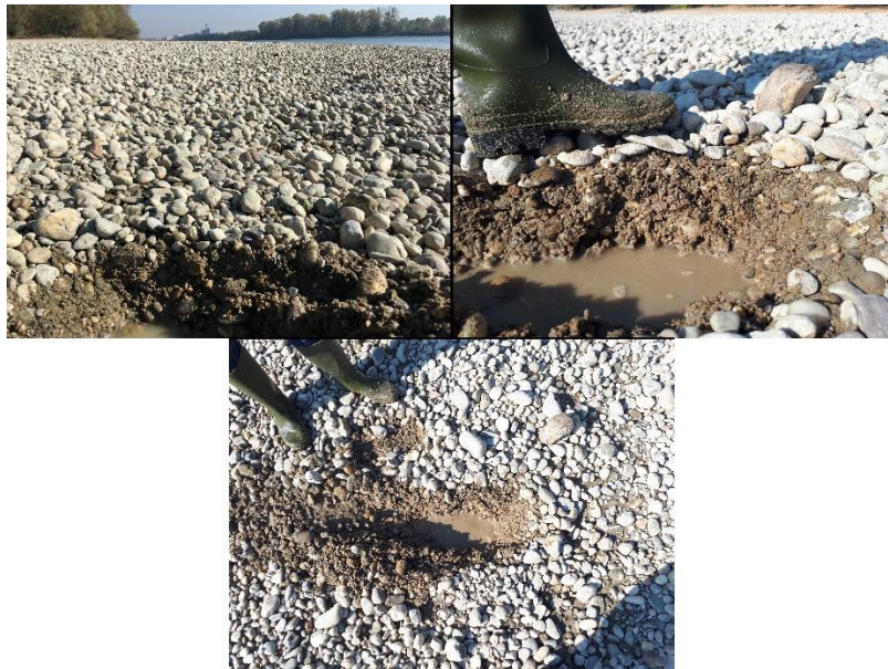
1076 Figure A2: Images of bed armouring, taken during our surveys in the Upper section of the Hungarian Danube. We 1077 broke the surface armour to showcase the presence of the underlying finer fractions. 1078
