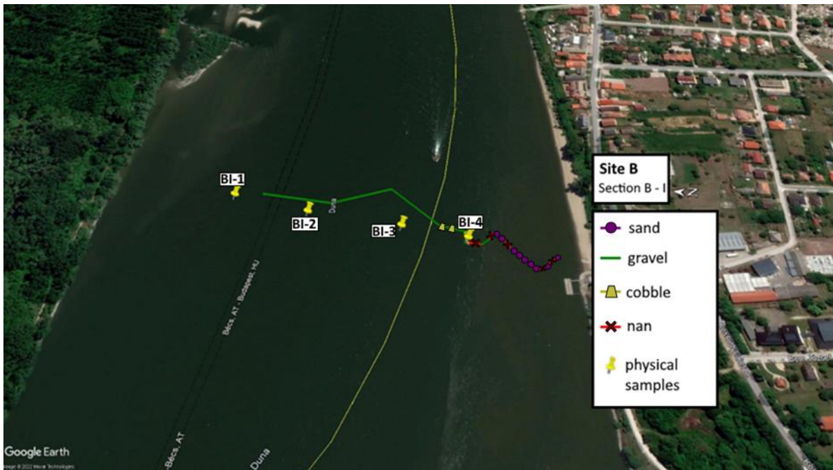
1124 1125 Figure E1: The path of the vessel and camera in Section B - I, Site B. The polyline is coloured based on the sediment 1126 seen during visual evaluation of the video. Yellow markers are the locations of physical bed material samplings. (Map 1127 created with Google Earth Pro)
