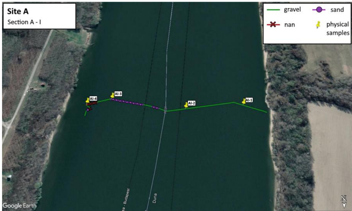
1086 Figure C1: The path of the vessel and camera in Section A - I, Site A. The polyline is coloured based on the sediment 1087 seen during visual evaluation of the video. Yellow markers are the locations of physical bed material samplings. (Map 1088 created with Google Earth Pro) 1089
