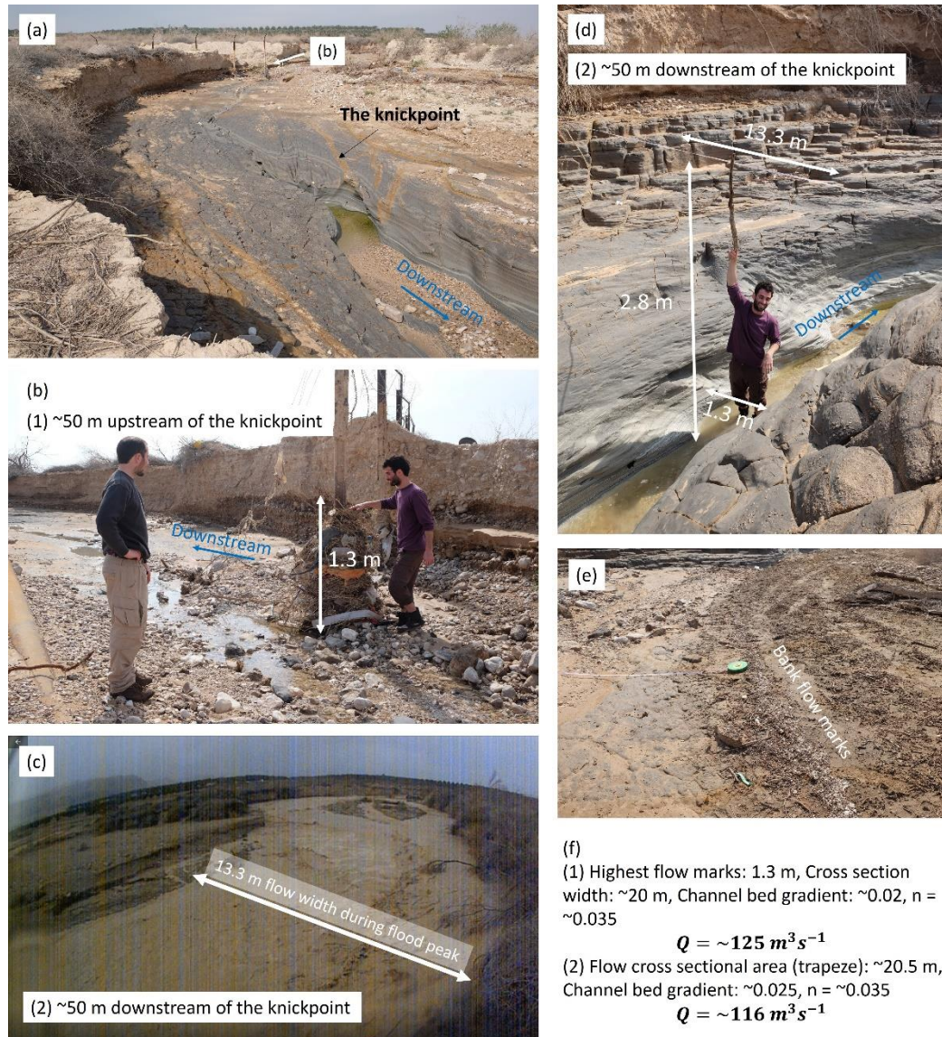
Figure S1: Reconstruction of the 27-Feb-2019 flood peak, the highest peak on our record (Fig. 8a). (a) The Nahal Og knickpoint (location is indicated in Fig. 2c) is incised into the lacustrine-laminated silt clay deposits of the shelf. (b) Measuring high watermarks on a metal pole located 50 m upstream the knickpoint. (c) TLC snapshot of the flood peak, looking upstream. The flow width during flood peak is indicated. (d) Estimation of the channel geometry using high flow marks that were left on the channel banks are shown in (e). (f) Calculation of the estimated peak discharge according to the parameters measured in the two locations.
