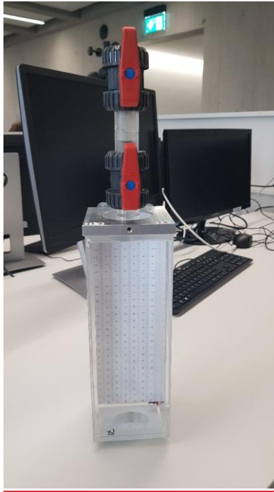
460 Figure 2: One of the six sedimentation chambers with the two ball valves on top. The walls are made of transparent Plexiglas, and on the back, wall can be seen the graph paper that is used as a visual reference for trajectory analysis of the sedimenting particles.
