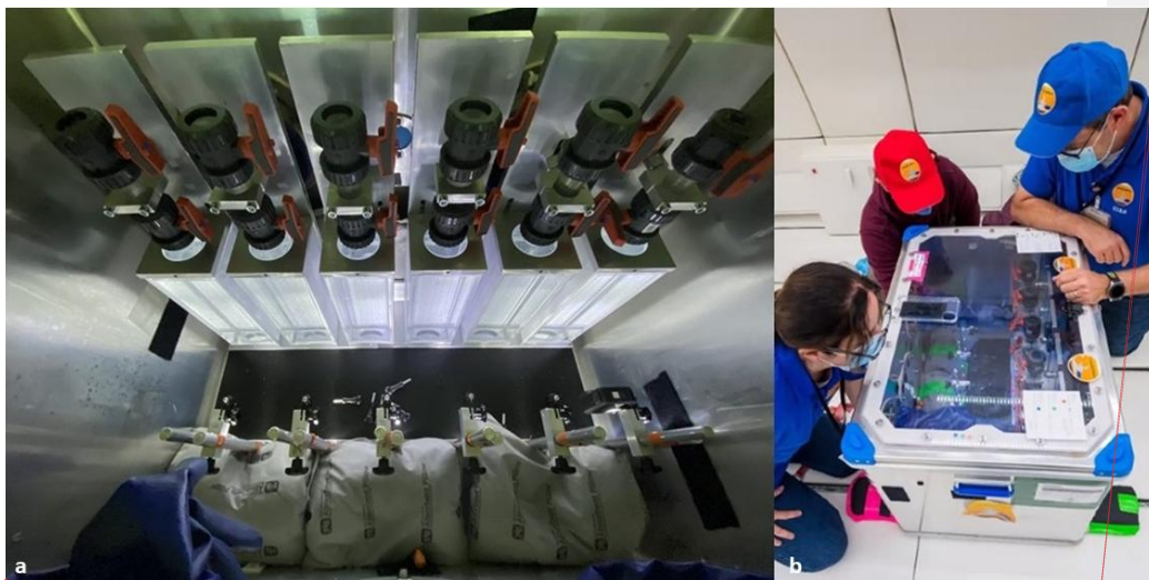
Figure 3-4: Left side (panel a) Top view of the experimental apparatus on board the 4th Swiss Parabolic Flight Campaign held in Dübendorf Zurich (June 2020), just before the flight. The six square tubes filled with water and each mounted by two ball valves inside the aluminum containing box are shown. In front of the settling chamber are GoPro cameras and LED lighting. Behind the GoPro, absorbent pillows in case of liquid leakage, are visible. Right side (panel b): The parabolic flight team as they maneuver and test the accessibility of the settling chamber using gloves inside the aircraft, the day before the parabolic flight. The team consists of four members, three of whom are visible in the figure. The blue-shirted team members, F. Trudu on the left and N. J. Kuhn on the right, flew and performed the experiments.
