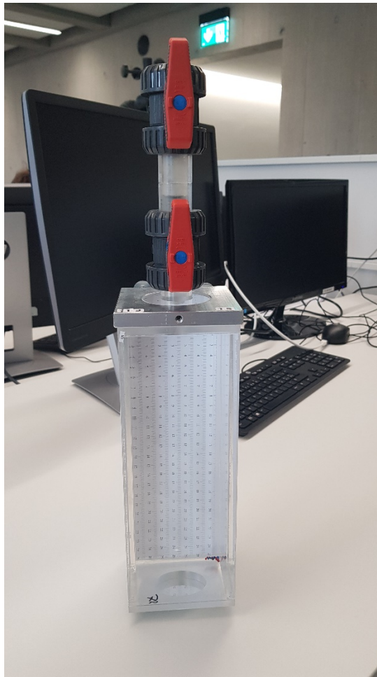
Figure 2: One of the six sedimentation chambers with the two ball valves on top. The walls are made of transparent Plexiglas, and on the back, wall can be seen the graph paper that is used as a visual reference for trajectory analysis of the sedimenting particles.
