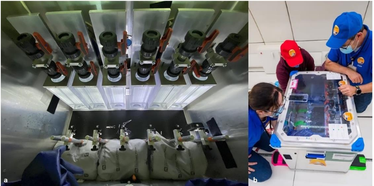
Figure 3: Left side (panel a) Top view of the experimental apparatus on board the 4th Swiss Parabolic Flight Campaign held in Dübendorf Zurich (June 2020), just before the flight. The six square tubes filled with water and each mounted by two ball valves inside the aluminum containing box are shown. In front of the settling chamber are GoPro cameras and LED lighting. Behind the GoPro, absorbent pillows in case of liquid leakage, are visible. Right side (panel b): The parabolic flight team as they maneuver and test the accessibility of the settling chamber using gloves inside the aircraft, the day before the parabolic flight. The team consists of four members, three of whom are visible in the figure. The blue-shirted team members, F. Trudu on the left and N. J. Kuhn on the right, flew and performed the experiments.
