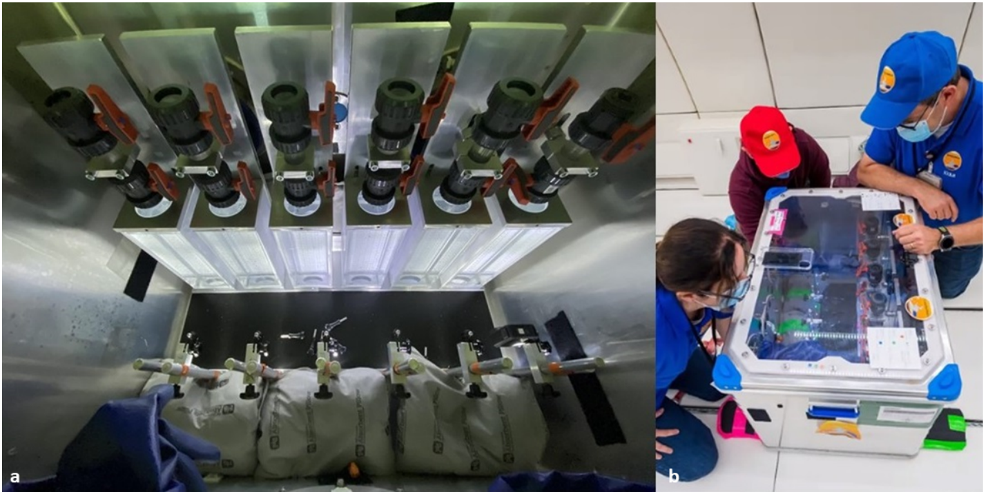
435 Figure 4: Left side (panel a) Top view of the experimental apparatus on board the 4th Swiss Parabolic Flight Campaign held in Dübendorf Zurich (June 2020), just before the flight. The six square tubes filled with water and each mounted by two ball valves inside the aluminum containing box are shown. In front of the settling chamber are GoPro cameras and LED lighting. Behind the GoPro, absorbent pillows in case of liquid leakage, are visible. Right side (panel b): The parabolic flight team as they maneuver and 440 test the accessibility of the settling chamber using gloves inside the aircraft, the day before the parabolic flight. The team consists of four members, three of whom are visible in the figure. The blue-shirted team members, F. Trudu on the left and N. J. Kuhn on the right, flew and performed the experiments.
