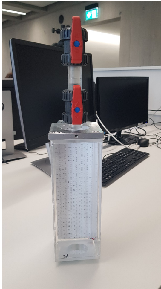
425 Figure 2: One of the six sedimentation chambers with the two ball valves on top. The walls are made of transparent Plexiglas, and on the back, wall can be seen the graph paper that is used as a visual reference for trajectory analysis of the settling particles. Image credit: B. Kuhn
