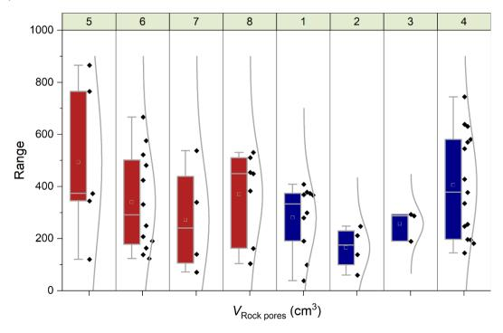
Figure 8: Chamber-specific box plots and distribution curves summarizing the volume of rock pores ( $V_{\text{Rock pores}}$ ) connected to each chamber determined during  $CO_2$  flux measurements. Boxes indicate the 25 % - 75 % range alongside the 1.5 interquartile ranges with mean (open square) and median (line). Panels at the top show the chamber identifiers (Table 1) and colors indicate the origin (Brusquet: red, sites 5 - 8; Moulin: blue, sites 1 - 4).
