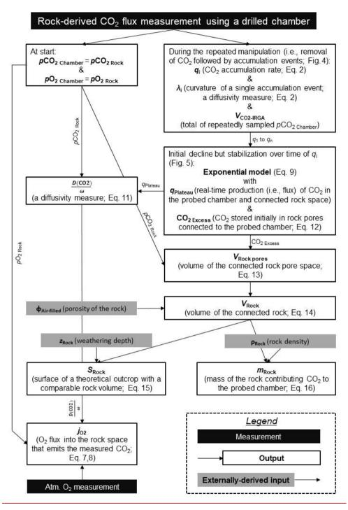
Figure B1: Central data-flow for the new approach developed in this study to quantify the diffusive exchange of CO<sub>2</sub> and O<sub>2</sub> during shallow rock weathering based on real-time measurements using drilled headspace chambers.
