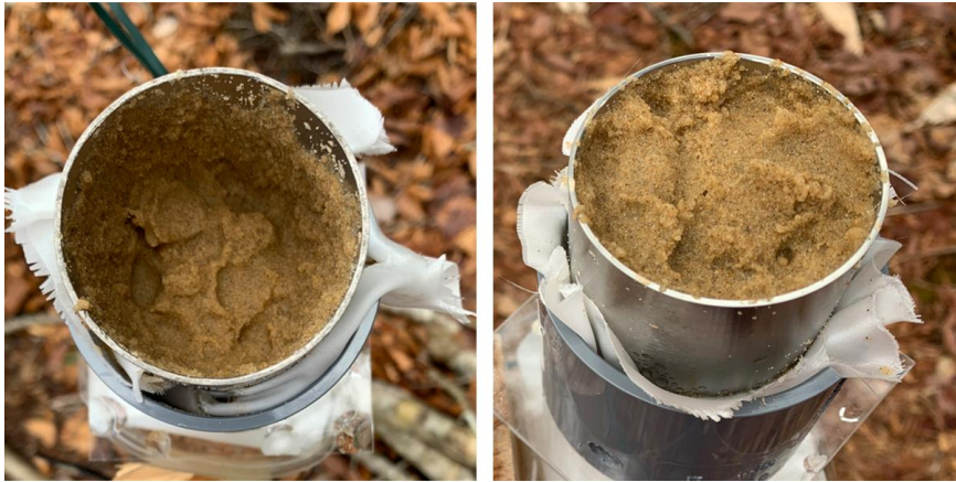
396 Fig. 1 Splash cups at the concentrated impact location (left) and at an exemplary general location (right)
